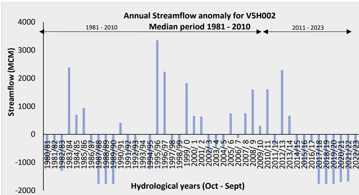
*Figure 4.4: Annual streamflow deviation from the long-term median at station V5H002.*
